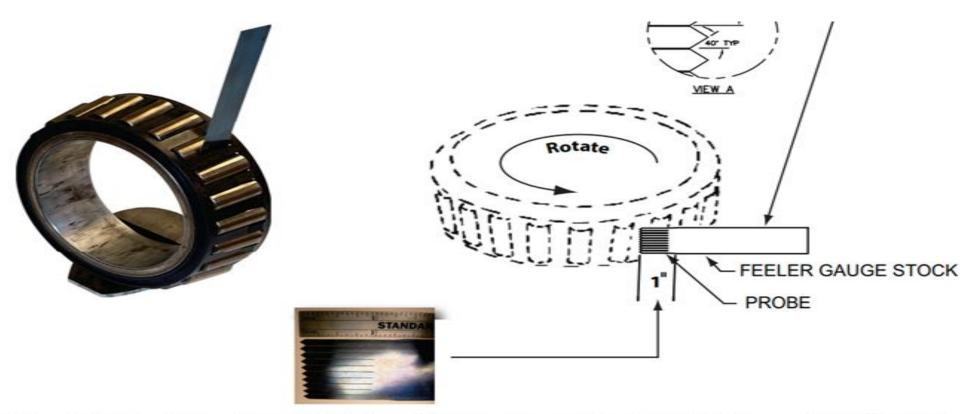
Place feeler of surface roughness tester between the roller and cage adjacent to both the large and small ribs, rotate inner ring. Any surface defects must be noted by roughness felt through the feeler gauge. Probes must be checked and replaced as tips wear to avoid loss of sensitivity.
